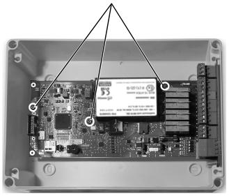
Fig. 6 PCB fixing screws
