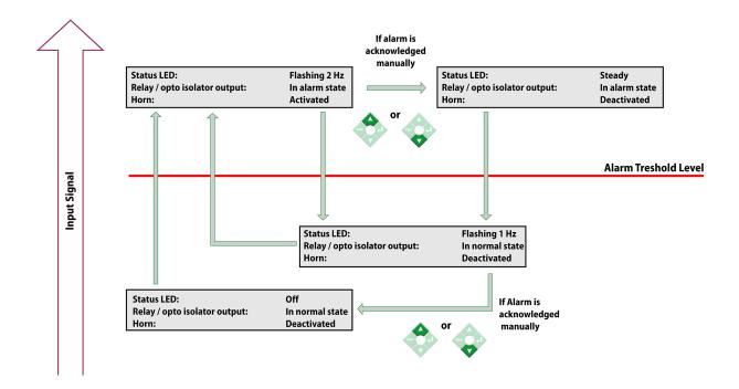
Fig. 12 2A - Automatic reset configuration with alarm memorisation
