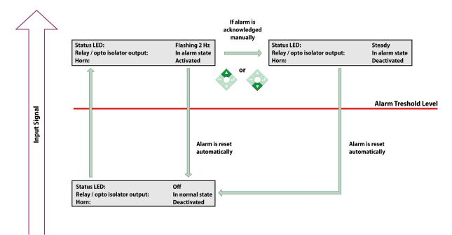
Fig. 10 1A - Automatic reset configuration
