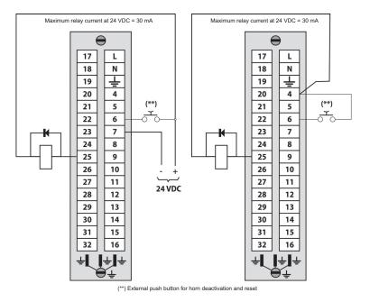
Fig. 9 "CAUTION" output connection to external relay and for button for remote acknowledgement and alarm reset
