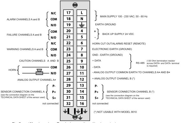
Fig. 7 19" rack version – Terminal connection with relay outputs
