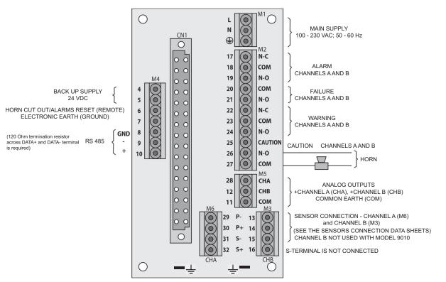
Fig. 8 Wall mounted version – Terminal connection
