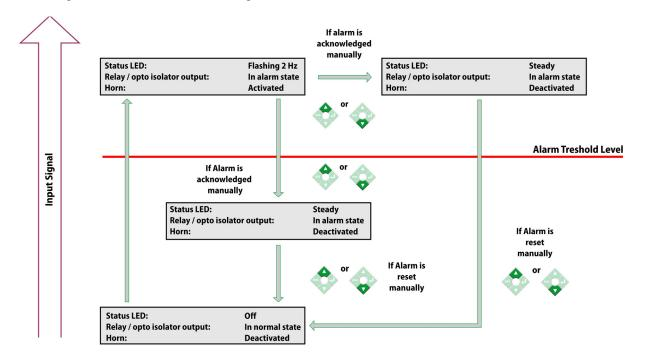
Fig. 11 1M - Manual reset configuration
