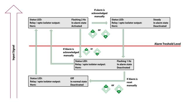
Fig. 13 2M - Manual reset configuration with alarm memorisation
