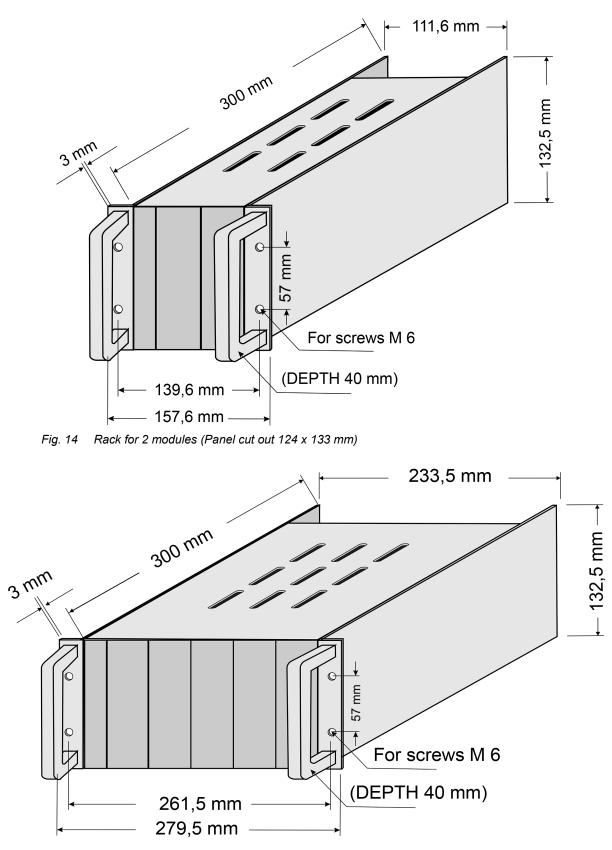
Fig. 15 Rack for 5 modules (Panel cut out 246 x 133 mm)
